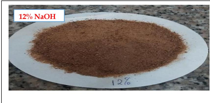
Figure 1: Untreated (raw), 6% and 12% NaOH-treated clay samples
