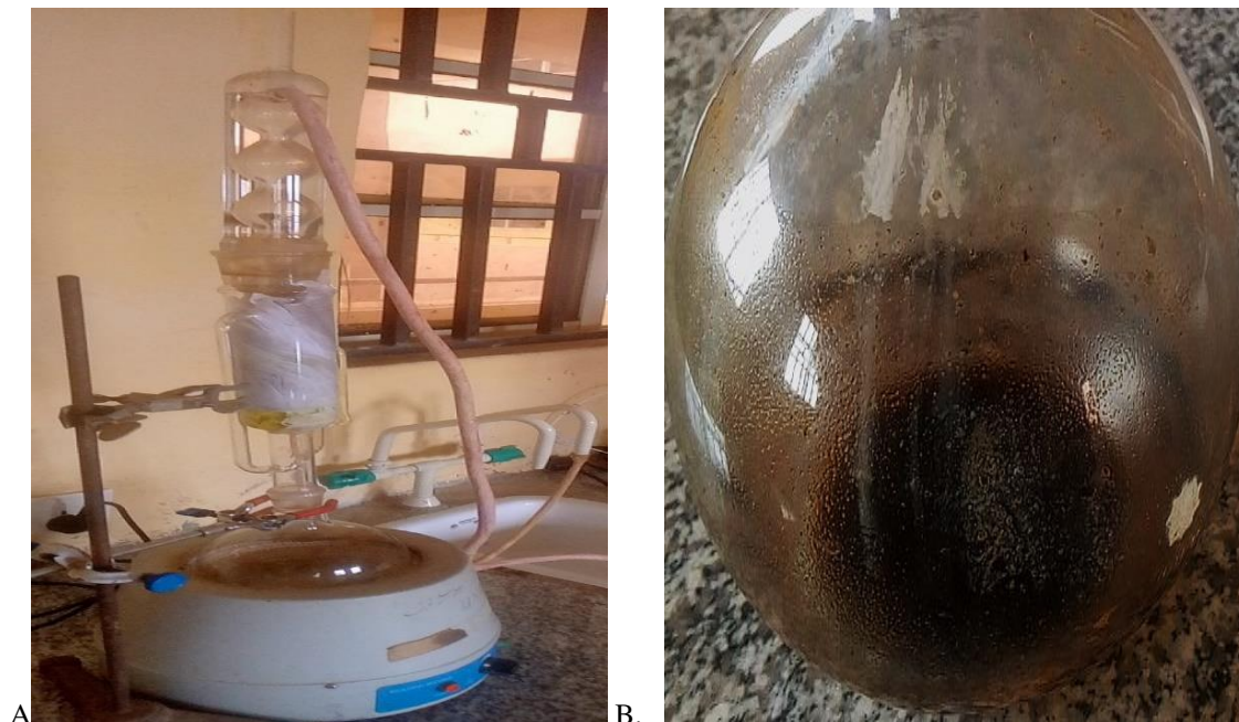
Plate 3: A and B showing the soxhlet extraction and the extraction product
